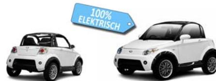
The **HR GTZero** is designed and a prototype is build by the Rotterdam University HR. This electric sport cabrio has two seats, a range of 130 km, a maximum speed of 100 km/hour and a enegyconsumption of 118Wh/km. Exterior dimensions are 3830 x 1480 x 1600 mm.(l x w x h) Acceleration 0...100 km/h in 15 seconds.
