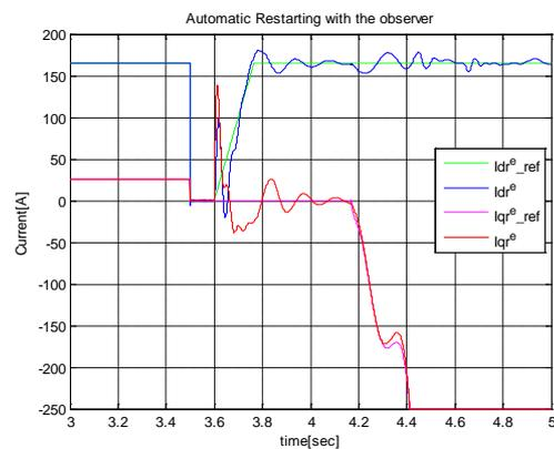
Figure 8: Simulated dq-axis currents with an adaptive observer
