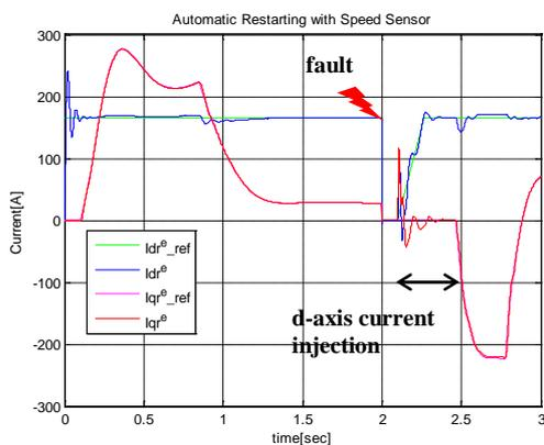
Figure 6: Simulated dq-axis currents with a speed sensor
