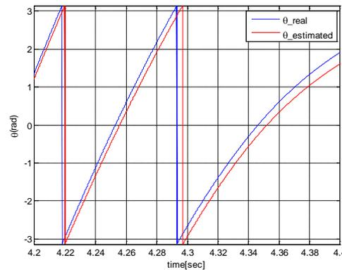
Figure 9: Simulated thetas in transient state with an adaptive observer
