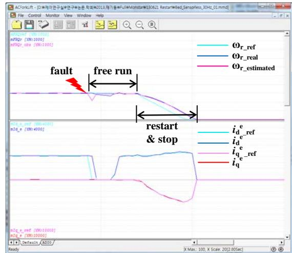
Figure 13: Speeds and dq-axis currents of a restarting method with an adaptive observer
