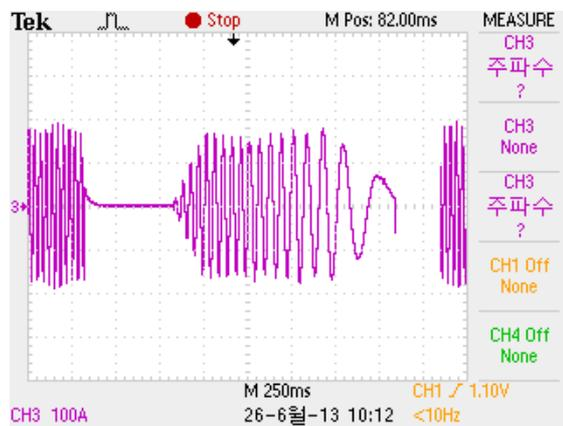
Figure 18: Phase current of a restarting method with a speed sensor in the forklift.
