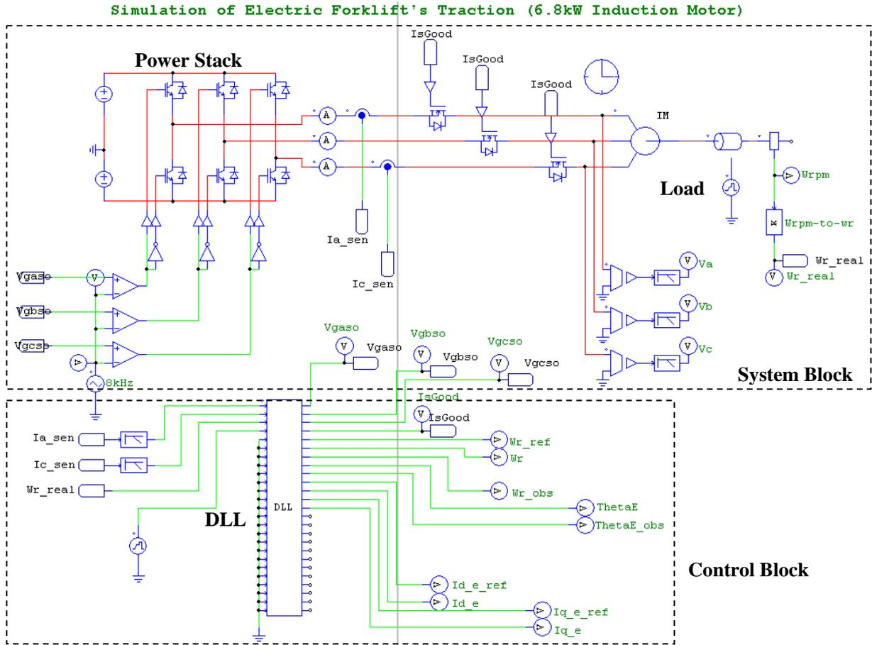
Figure 4: Block diagram for simulation
