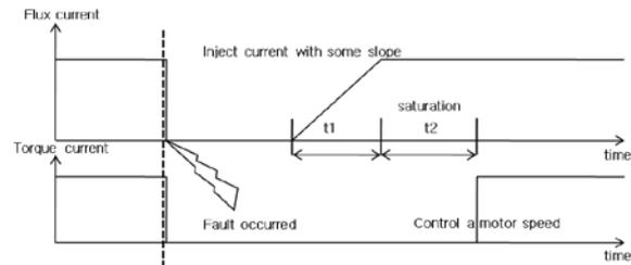
Figure 2: Injecting flux and torque currents with a measured rotor speed
