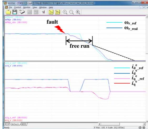
Figure 17: Speeds and dq-axis currents of a restarting method with a speed sensor in the forklift.
