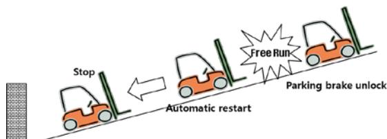
(b) Case 2. Parking brake is unlocked on a slope
