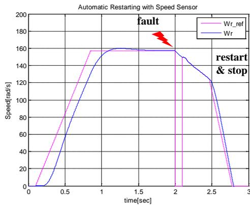
Figure 5: Simulated speeds with a speed sensor
