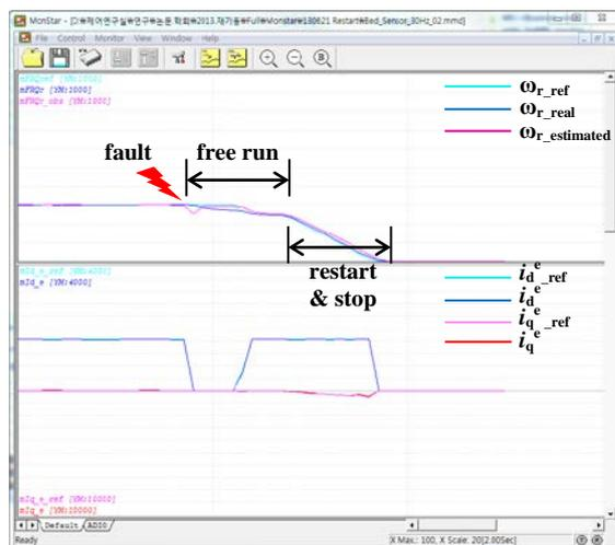
Figure 11: Speeds and dq-axis currents of a restarting method with a speed sensor
