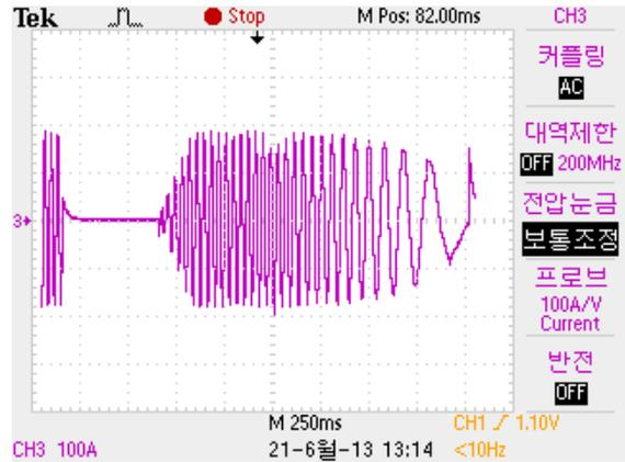
Figure 12: Phase current of a motor
