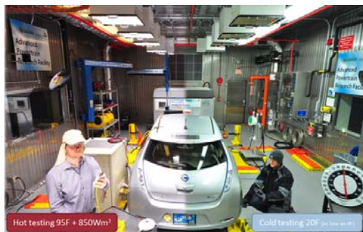
Figure 5: BEV testing displayed at 95°F with solar emulation on the left and testing at cold ambient temperatures on the right (ANL facility)
